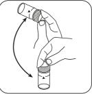
Dissolve tablet(s) by inverting.
