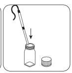
Swirl around to dissolve the Keep the UV lamp in the sample. Note: wear UV safety goggles!
