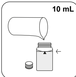
Fill 24 mm vial with 10 mL sample .
