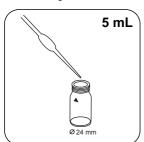
Put 5 mL sample and 5 mL of deionised water in the sample vessel.
